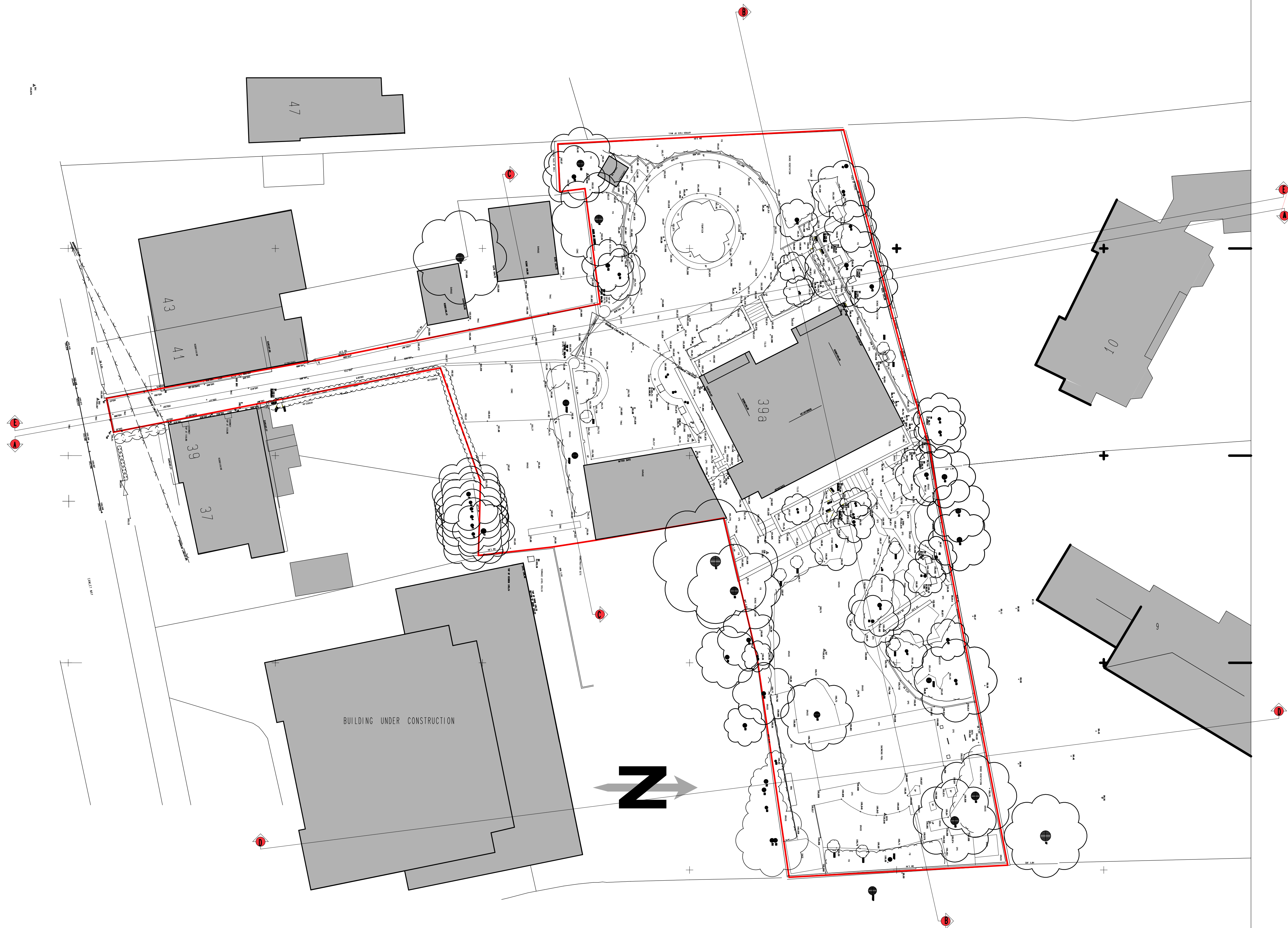
EXISTING SITE PLAN (1:200) EXISTING HARD STANDING ON SITE INCLUDING EXG BUILDINGS/ ACCESS ROAD - 1050M2
